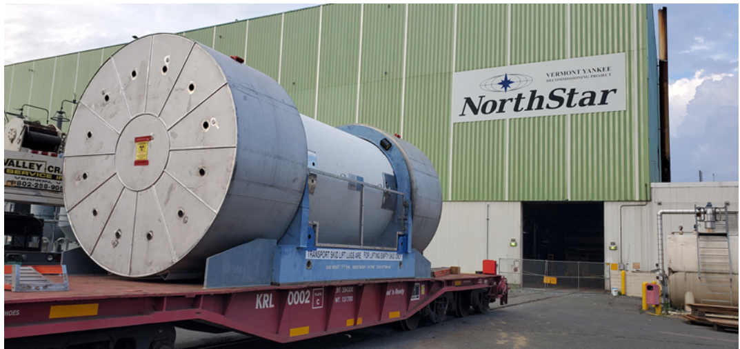
Orano's MP197HB transport cask prepared for shipping segmented waste to disposal in West Texas.
