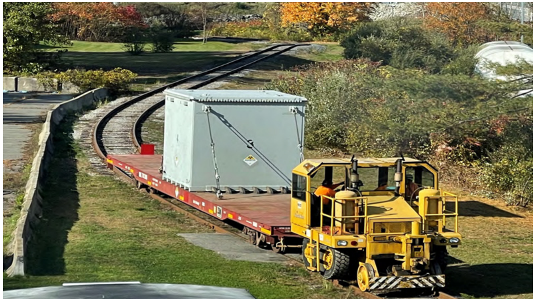
Final disposal cask leaves the site with the last pieces of the segmented Vermont Yankee reactor.
